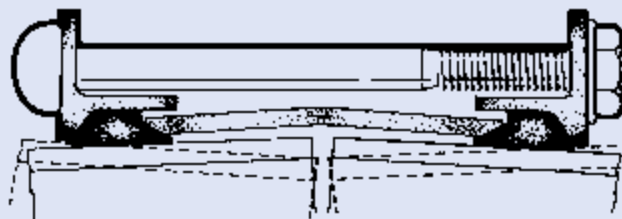
Flexible gasket and centre sleeve clearance allows angular movement.
