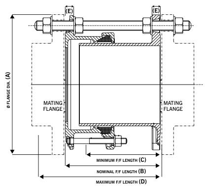
Note: Maximum Longitudinal F/F Adjustment = Maximum F/F Length - Minimum F/F Length
