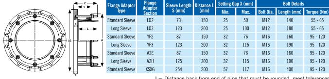
L= Distance back from end of pipe that must be rounded, meet tolerances, and free from any wrapping to ensure correct assembly.
