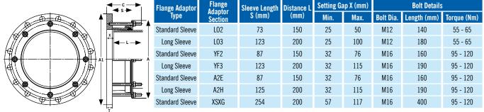
L= Distance back from end of pipe that must be rounded, meet tolerances, and free from any wrapping to ensure correct assembly.
